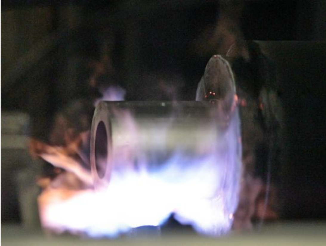
Above, Heat blasts the end of a roller as it's run through a roll forming machine. Left, Pierce Industries, on Paul Road in Chili. (Photo: SHAWN DOWD/@sdowdphoto / STAFF PHOTOGRAPHER)
